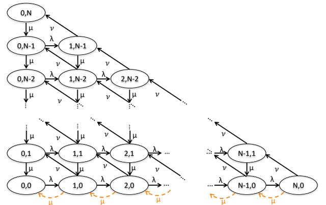
Fig. 2. Markov chain of a SCMS-PS station. The orange transitions exist only for the IP scenario.
