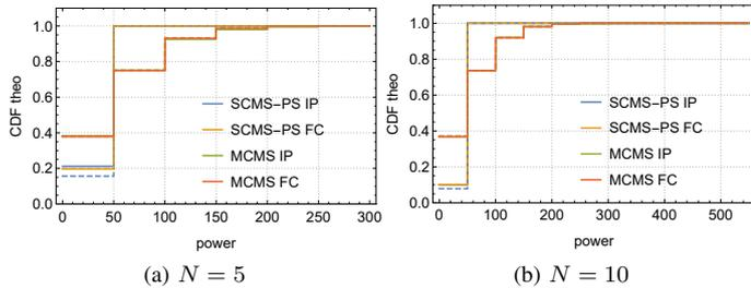
Fig. 7. CDF of charging power for  $\lambda = 8$ . The solid lines represent model predictions, the dashed lines simulation results.
