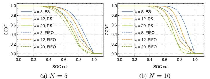
Fig. 6. CCDF of the SoC value for SAEVs leaving the charging station.
