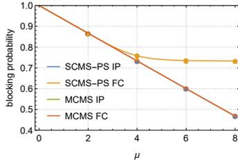
Fig. 4. Blocking probability versus customers' arrival rate for  $\lambda = 15$  vehicles/hour and  $N = 10$ . Curves for SCMS-PS and SCMS are overlapping. Points show the simulations results. Triangles refer to the SCMS case.
